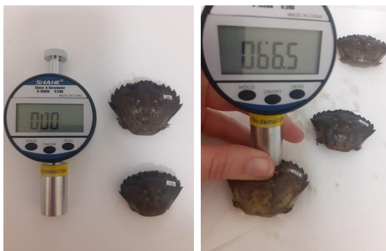
Figure 8: SHORE A durometer and placement on the crab shell
