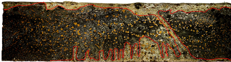
FIGURE F.1: Specimen 3.0%-300-8: chlorides ingress from the side of the bottom surface (penetration depth of chloride ions in lighter part).
