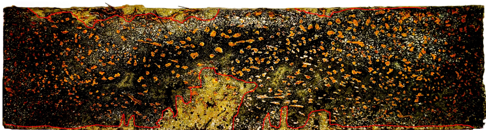
FIGURE F.2: Specimen 3.0%-300-9: chlorides ingress from the side of the bottom surface (penetration depth of chloride ions in lighter part).
