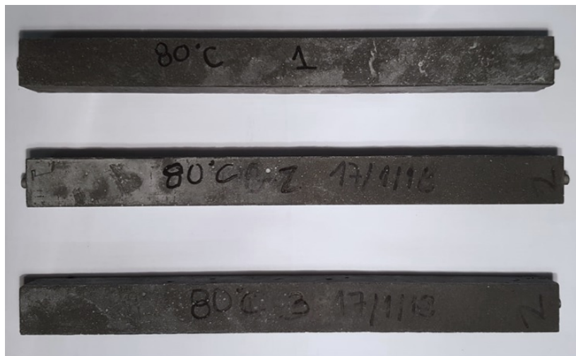
FIGURE 4.9: UHPC specimens set 1 after long term ASR test.
