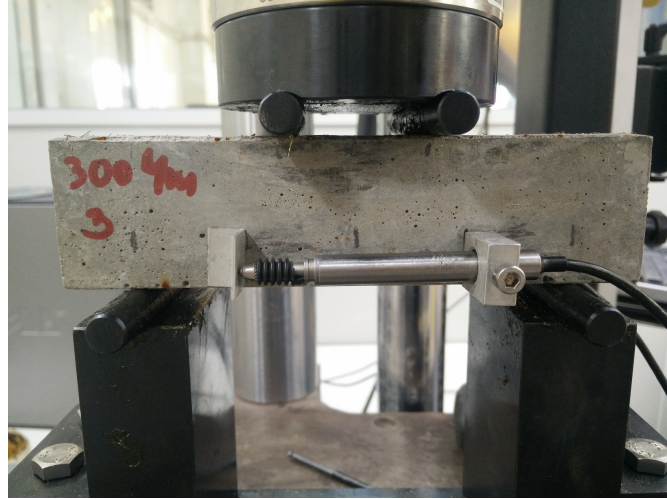
FIGURE 5.1: Four-point bending test configuration and positioning of the LVDTs on the lateral surface of the prism.
