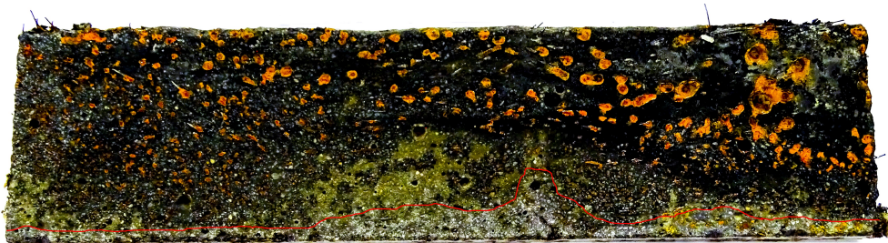
FIGURE F.5: Specimen 3.0%-350-6: chlorides ingress from the side of the bottom surface (penetration depth of chloride ions in lighter part).
