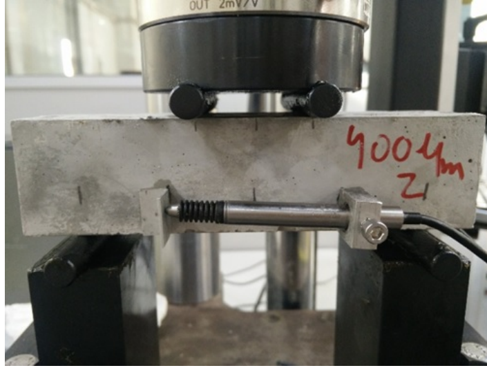
FIGURE 6.2: Four point bending test.
