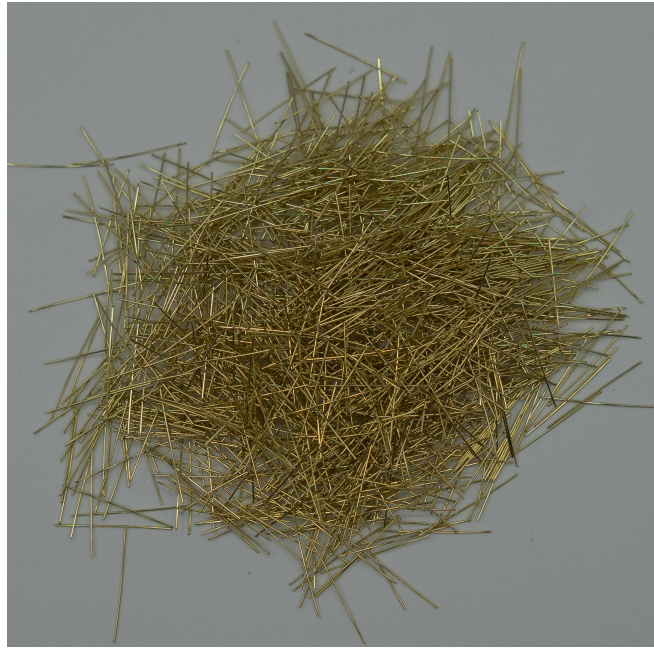
FIGURE 3.1: Steel fibres employed to produce UHPFRC.
