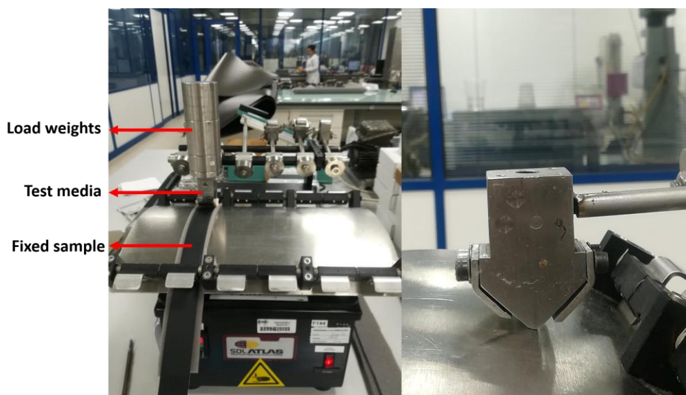
Figure 18 On the left, the arrangement for abrasion tests in Gakushin ; on the right, the triangular test media used.
