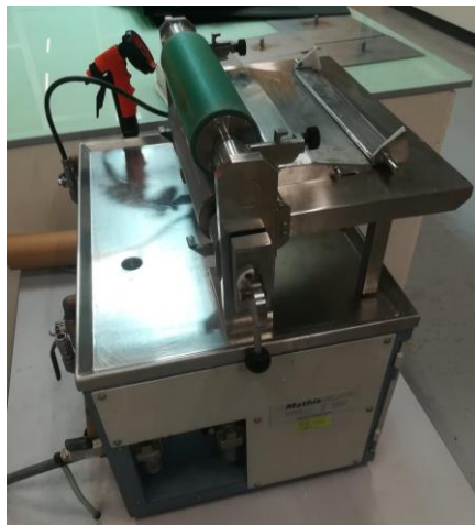
Figure 10 MATHIS, equipment for lacquering simulation in laboratory.
