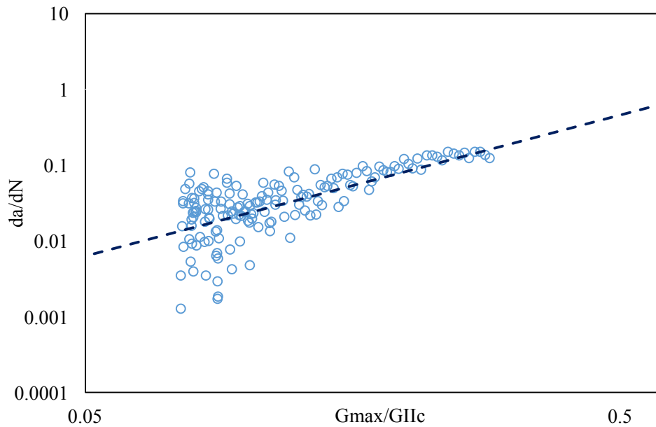
Figure 19 - Paris law curve for pure mode II
