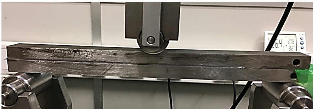
Figure 9 - Outline of the ENF test setup
