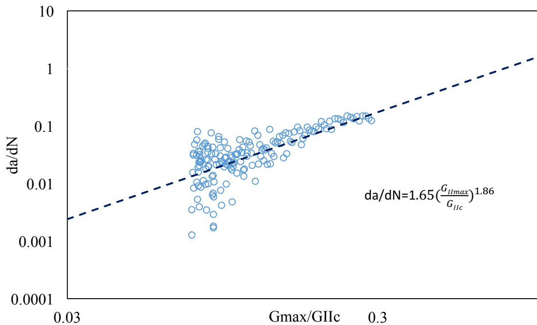
Figure 10 – A typical Paris law curve
