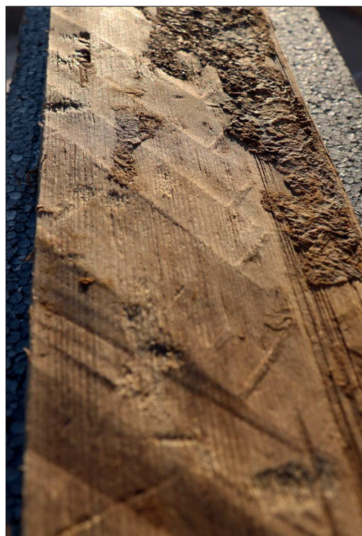
Fig. 12. Condition of the uncovered barrel staves with traces of planing and residue (Photo: Bence Simon).
