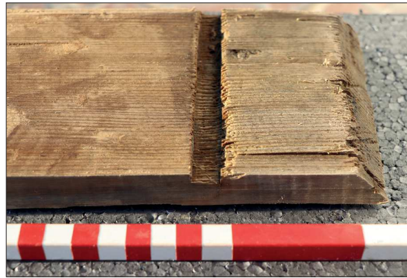
Fig. 13. End of a staff with the croze groove in perfect condition (Photo: Bence Simon).
