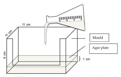
Figure 2.1.3-2: A schematic drawing of the mold for agar herbicide plates.
