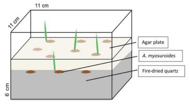
Figure 2.1.3-3: Structure of the agar test: 1st layer = agar plate consisting of agar, herbicide and nutrients; 2nd layer = pre-germinated A. myosuroides seeds; 3th layer = fire-dried quartz sand.
