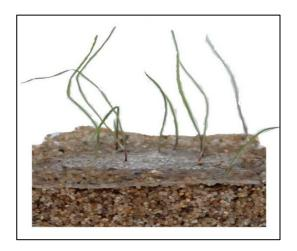
Figure 2.1.3-4: Structure of the agar test: 1st layer = fire-dried quartz sand; 2nd layer = pre-germinated A. myosuroides seeds; 3rd. layer = agar plate consisting of agar, herbicide and nutrients. Plants showed in the picture are from the sensitive standard treated with no herbicide, 7 days after transplanting.
