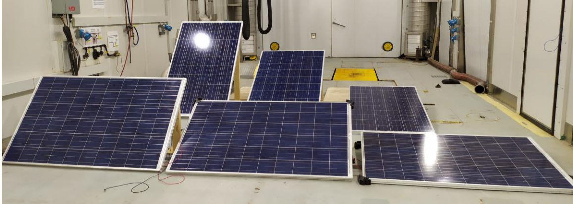
Figure 4.3. Solar PV array setup for validation test.
