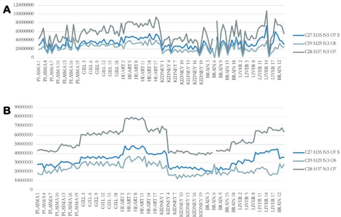
Figure 1. Instrumental Variation Corrected Using Internal Standards. Standard mix contained five peptides, 3 of which were used for normalization. 2uL of internal standards were spiked into each sample. Peak integration and area were found using MassHunter Qual. (A) Peak intensity before normalization, and (B) Peak intensity after normalization.
