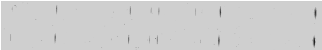
Figure 2.6 Shown are two exposures from a Pt/Ne HCL on a photographic plate. The wavelength range is approximately 1505 - 1550 \text{ \AA} with a dispersion of 0.044 \text{ \AA pixel}^{-1} . Note that the bottom track is shifted to the left of the top track due to the plate holder moving between exposures.
