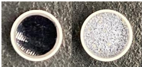
Fig. 51. Photos of TGA sample geometry. Disc on the left and powder on the right.
