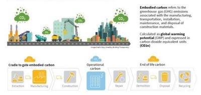
Figure 71: Graphic defining and illustrating elements of embodied carbon. Source: U.S. General Services Administration (GSA)
