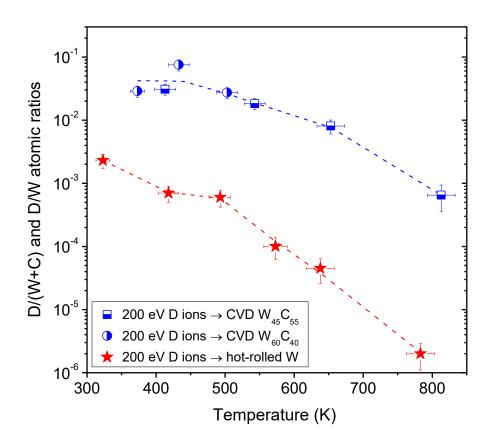
Figure 5. Deuterium concentration in the bulk of CVD tungsten carbide coatings and hot-rolled tungsten samples exposed to low-energy (about 200 eV/D) deuterium plasma to a fluence of about  $2\times10^{24}$  D/m<sup>2</sup>, as a function of the exposure temperature.
