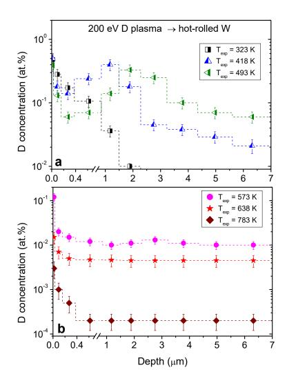
Figure 2. Depth profiles of deuterium trapped in hot-rolled W samples exposed to low-energy (about 200 eV/D) deuterium plasma to a fluence of about  $2\times10^{24}$  D/m<sup>2</sup> at temperatures in the range from 323 to 493 K (a) and in the range from 573 to 783 K (b). Please note that the scales of the ordinate axes on panels (a) and (b) are different.
