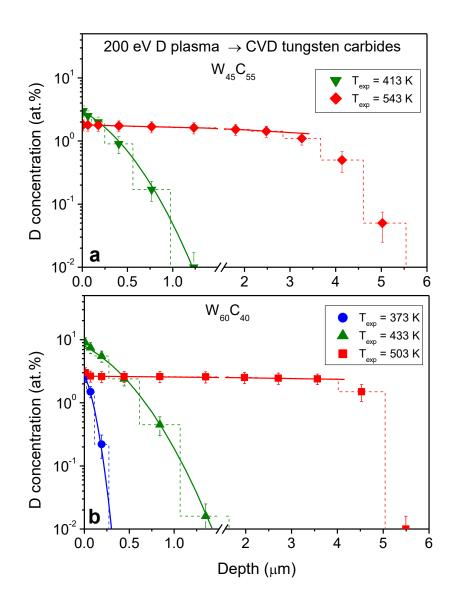
Figure 6. Measured (symbols) and calculated in accordance with Eq. (1) (solid lines) depth distributions of deuterium concentration in CVD tungsten carbide coatings  $W_{45}C_{55}$  (a) and  $W_{60}C_{40}$  (b) exposed to low-energy (about 200 eV/D) deuterium plasma to a fluence of about  $2\times10^{24}$  D/m<sup>2</sup> at various temperatures.
