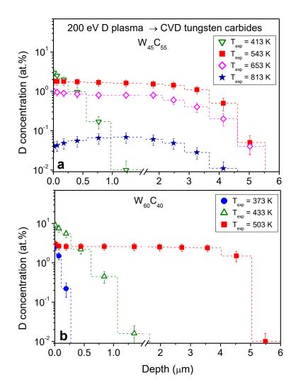
Figure 1. Depth profiles of deuterium trapped in CVD tungsten carbide coatings  $W_{45}C_{55}$  (a) and  $W_{60}C_{40}$  (b) exposed to low-energy (about 200 eV/D) deuterium plasma to a fluence of about  $2\times10^{24}$  D/m<sup>2</sup> at various temperatures
