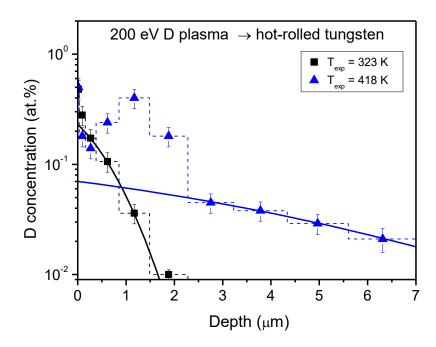
Figure 7. Measured (symbols) and calculated in accordance with Eq. (1) (solid lines) depth distributions of deuterium concentration in hot-rolled tungsten samples exposed to low-energy (about 200 eV/D) deuterium plasma to a fluence of about  $2\times10^{24}$  D/m<sup>2</sup> at temperatures of 323 and 418 K.
