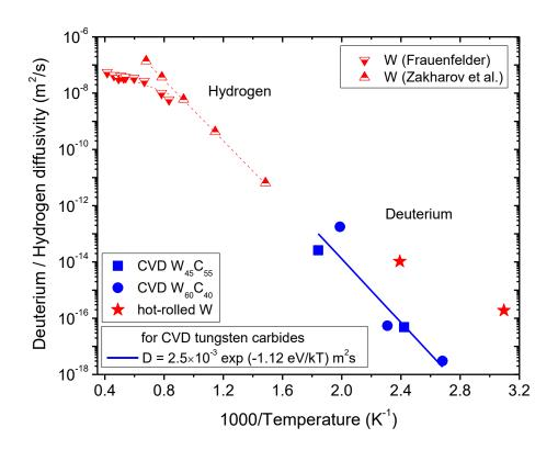
Figure 8. Comparison of the Arrhenius relations for the diffusion coefficients of deuterium in CVD tungsten carbide coatings  $W_{45}C_{55}$  and  $W_{60}C_{40}$ , as well as in hot-rolled tungsten samples, estimated in this work. In addition, the data on the diffusion of hydrogen (protium) in tungsten, taken from Frauenfelder [32] and Zakharov at al. [33], are also plotted.
