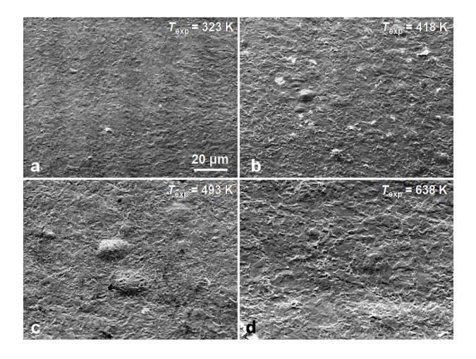
Figure 4. SEM images of surfaces of hot-rolled tungsten samples exposed to low-energy (about 200 eV/D) deuterium plasma to a fluence of about  $2\times10^{24}$  D/m<sup>2</sup> at 323 K (a), 418 K (b), 493 K (c), and 638 K (d). The scale bar given in panel (a) is valid for all images. The surfaces were tilted by 45°.
