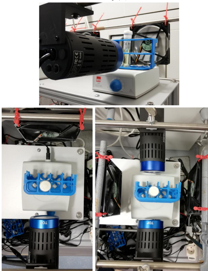
Figure 5.5. Configuration of the experimental setup using one or two LED lamps.
