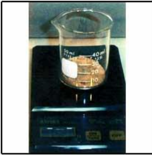
1. Weigh sample into tared beaker (5 grams of soil)
