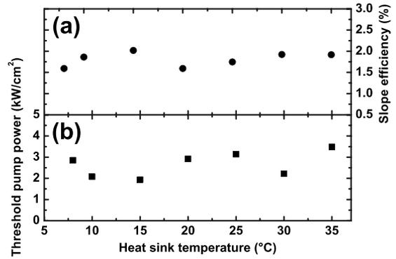
FIG. 2. (a) Slope efficiency of the VECSEL and (b) threshold pump power both measured with copper heat sink set to different temperatures.
