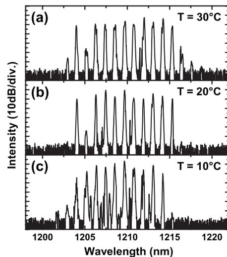
FIG. 3. [(a)–(c)] Laser spectra of the VECSEL recorded at a medium pump power level of 30 kW/cm<sup>2</sup> with heat sink set to different temperatures.
