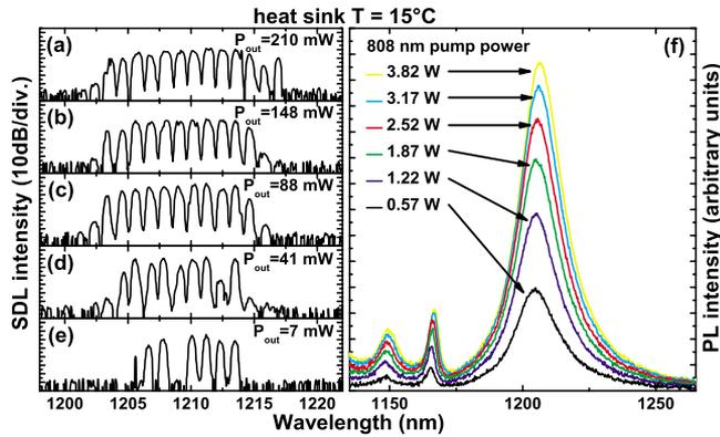
FIG. 4. (Color online) [(a)–(e)] Laser spectra recorded at different output power levels with heat sink temperature set to 15 °C. (f) PL spectra recorded in a different VECSEL setup at different pump-power levels below lasing threshold.
