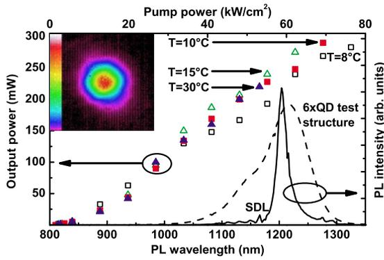
FIG. 1. (Color online) Left and top axes: light output characteristics with heat sink set to different temperatures. Right and bottom axes: PL of sixfold QD test structure and surface PL of QD VECSEL excited at 532 nm with excitation densities of 300 and 30 W/cm<sup>2</sup>, respectively. Inset: spatial intensity profile of the output beam recorded at 170 mW output power.
