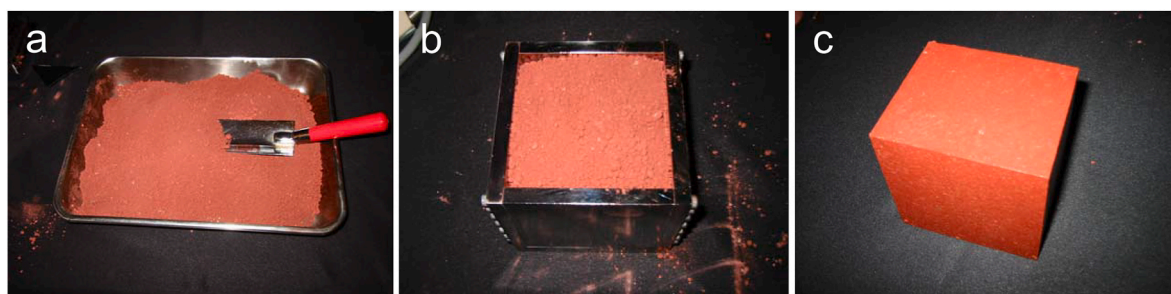
Fig. 9. (a) Bentonite clay with silica sand were cold-pressed in different states (b), producing powder compacts (c). Images reprinted by permission from Springer Nature CCC: V. Badescu (Ed.), Mars (2009) 543–50, Ishikawa [134] copyright 2009.
