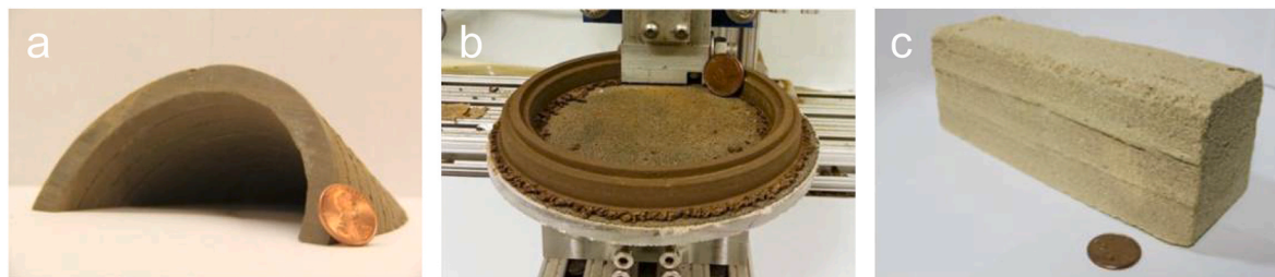
Fig. 20. Contour crafting of (unspecified) Martian regolith simulant with sulfur, producing (a) Martian regolith dome, (b) extruded sample with a smooth surface and (c) sample with large layers. Images reprinted with permission from Rapid Prototyping Journal 22 (2016) 848–856, Khoshnevis et al. [170], copyright Emerald Publishing Limited all rights reserved.
