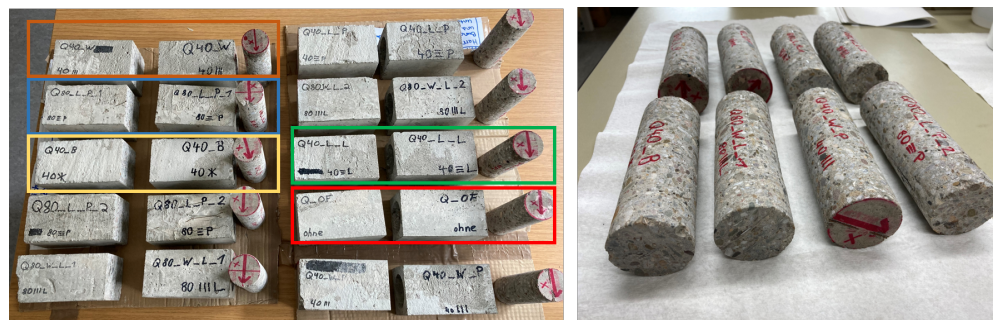
Figure 3. Photograph of the cast prismatic specimens (following being cut halfway along their length) and the extracted cylindrical sub-samples (left). The samples discussed in further detail are color-coded. Close-up on a selection of cylindrical sub-samples (right).
