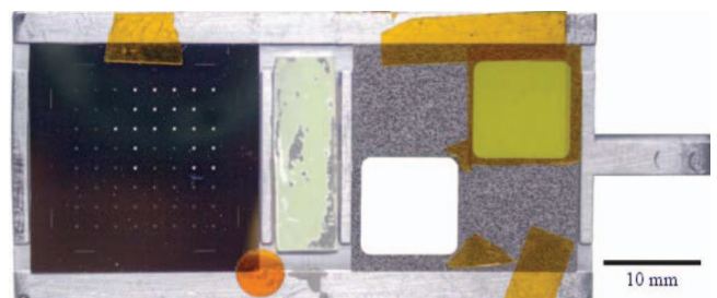
FIG. 5. Photograph of a sample holder with one multi-window sample (left), one adapter plate for smaller samples (right), and a fluorescence screen (center).
