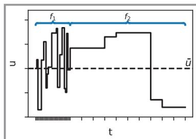
**Figure 2.** Frequency and amplitude modulated pseudo-random binary signal with 30 samples at  $f_1$  and 10 samples at  $f_2$ .  $f_1 \gg f_2$ . The input signal is sampled around the given mean  $\bar{u}$ .
