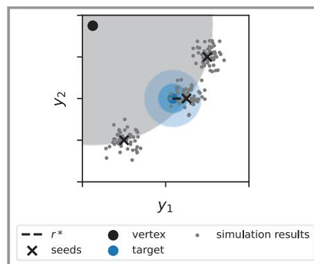
**Figure 5.** Phase 3 candidate selection. The vertex defines the selection of seeds, for target calculation. Size and number of simulation results inside the blue  $n$ -balls are used in the scoring function.
