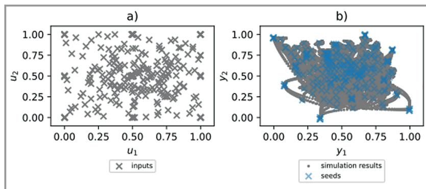
**Figure 7.** Results of the adaptive sampling algorithm for the CAE model. a) Two-dimensional control space representation for  $j$  ( $u_1$ ) and  $T_{in}$  ( $u_2$ ). b) Seeds and simulation results of the output space.
