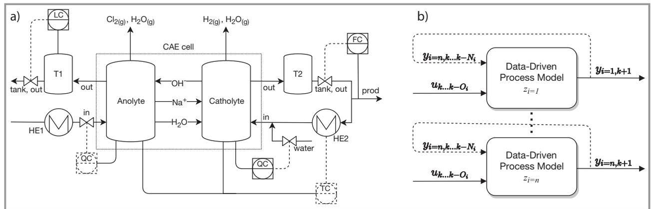
**Figure 6.** Model overview: a) Flowchart of chlor-alkali process model, dashed controllers are removed from model and associated manipulated variables are used as input variables in sampling algorithm. b) Structure of used recurrent neural networks. Each output is modeled separately. Parameters  $N$  and  $O$  are determined in hyperparameter tuning.
