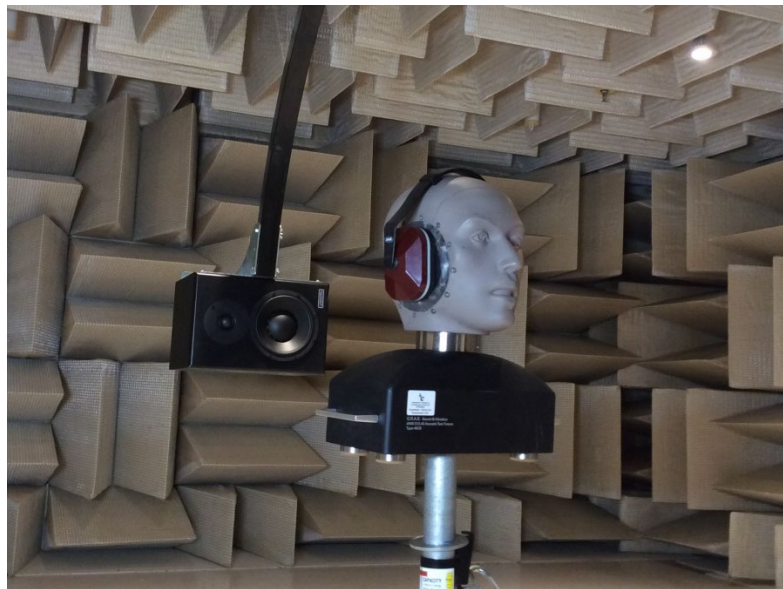
11 Figure 7 : Experimental set-up, sound source revolving around an ATF with the right ear 12 instrumented and protected with a modified EAR1000 earmuff
