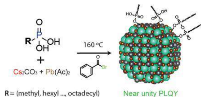
Scheme 1. Colloidal synthesis approach of CsPbBr 3 NCs employing only PA surfactant.
