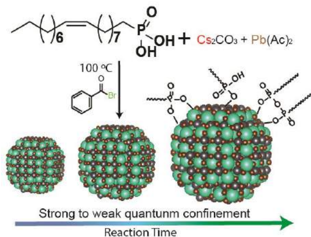
Scheme 1. Colloidal approach to obtain CsPbBr 3 NCs employing oleylphosphonic acid.
