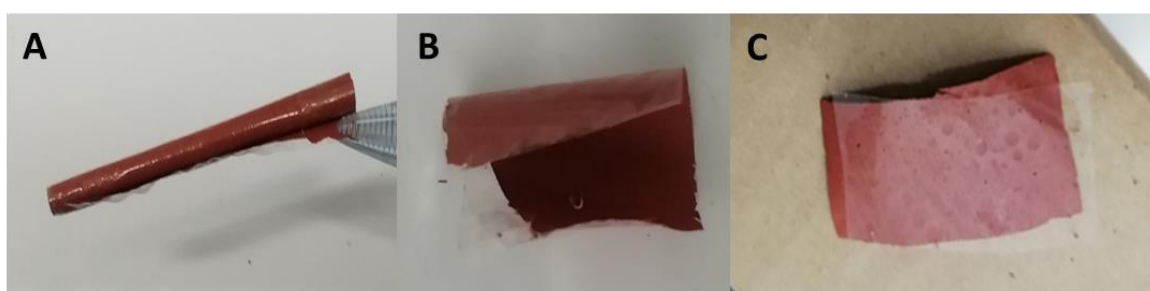
Figure 4.28 – Examples of Fluorinated Ethylene Propylene (FEP, 25 \mu\text{m} ) covered with conductive coating. A and B correspond to stable adhesion, C to unstable one.
