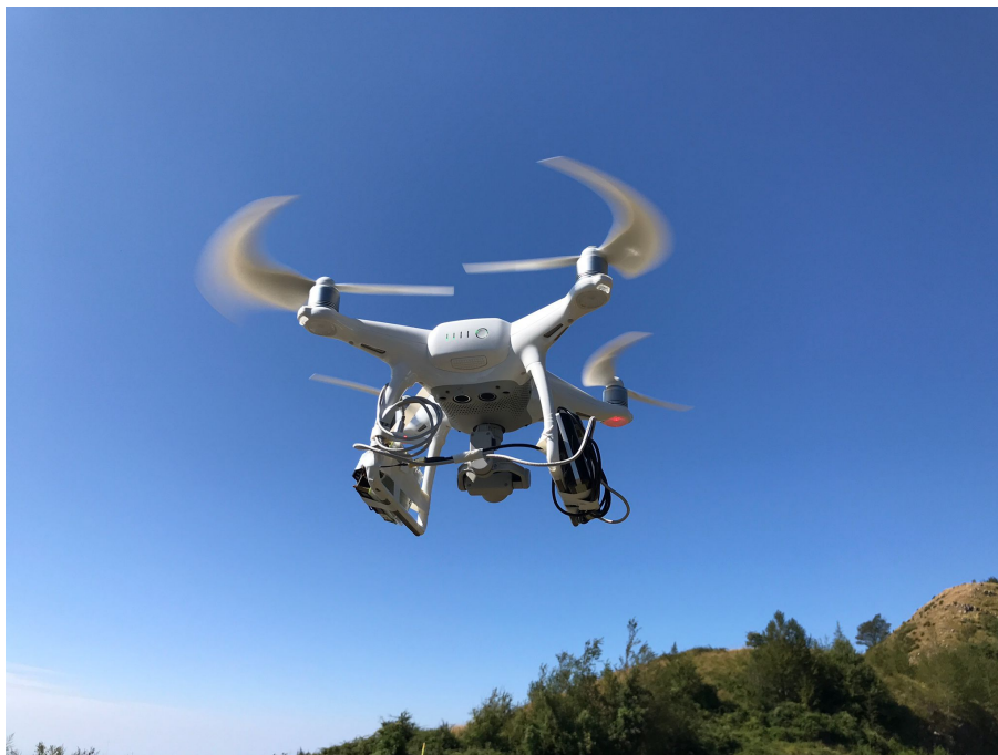
Figure 5.7: UAV equipped with our IoT LoRaWAN gateway
