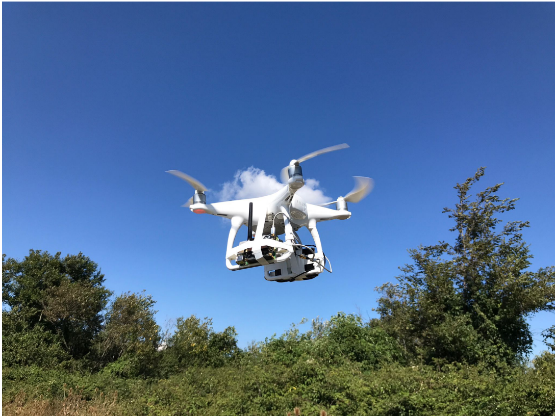
Figure 6.10: Flying drone with LoRa gateway on-board
