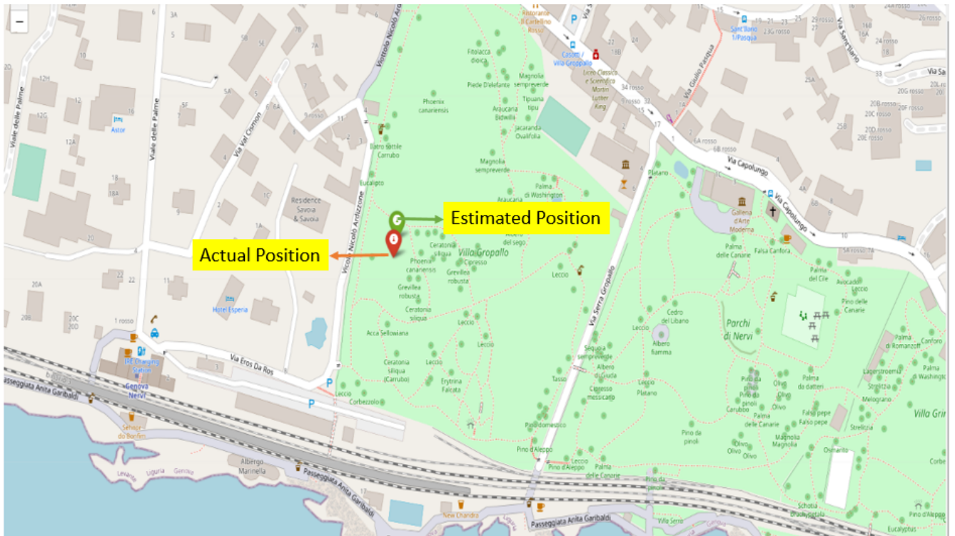
Figure 6.9: The position of the actual sensor (red marker) and the estimated position of the sensor (green marker) using trilateration algorithm.
