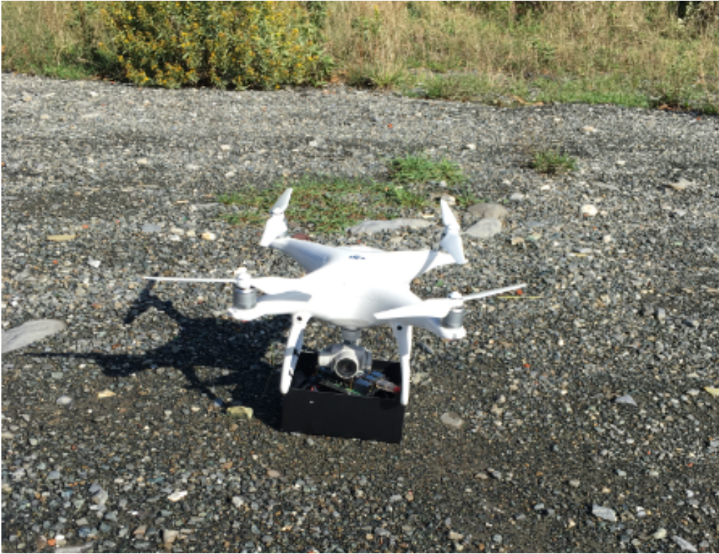
Figure 4.4: UAV equipped with the IoT gateway
