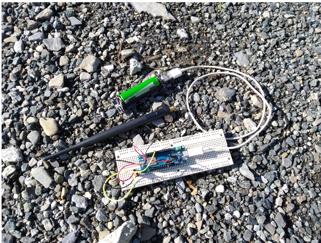
Figure 4.3: IoT devices based on Arduino MKR WAN 1300
