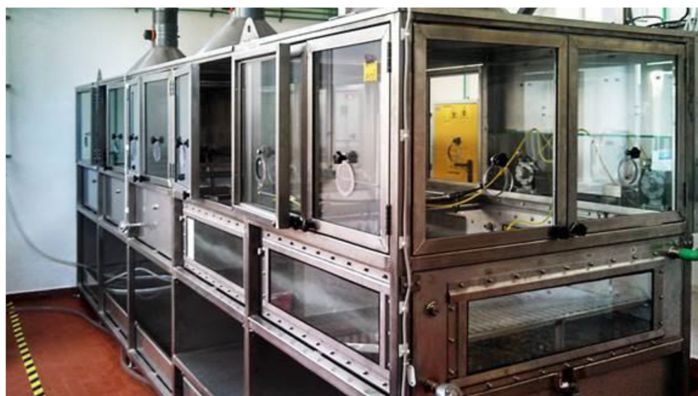
Figure 5. Pilot tank device for oil-adsorbent capacity testing of Grafysorber ® G+ and PP booms in dynamic conditions.
