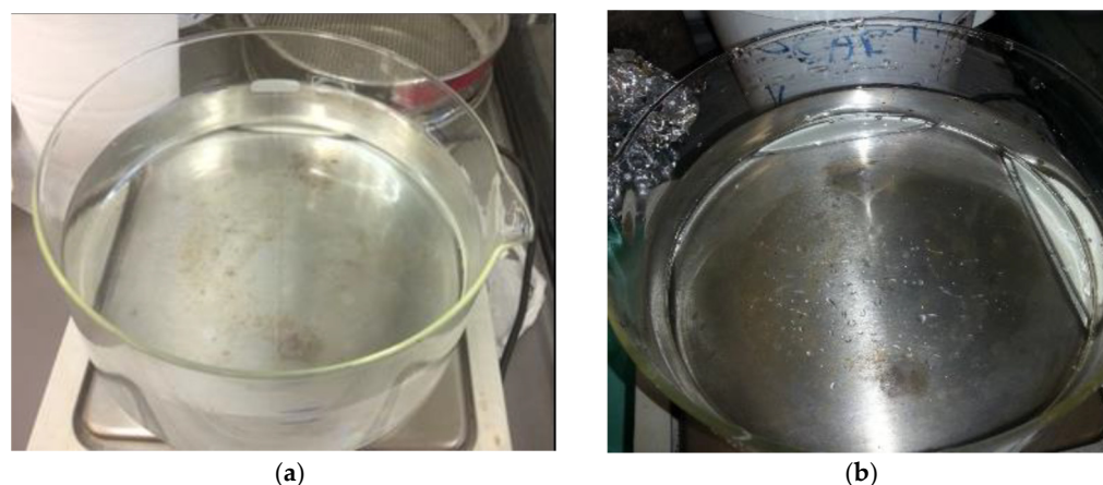
Figure 9. Water appearance after test n.3 with a thin film of diesel using (a) Grafysorber® G+; (b) PP.
