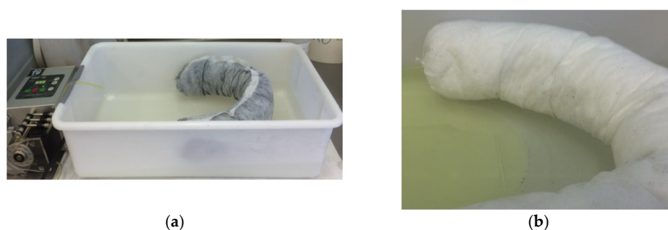
Figure 7. Experimental device for containment tests: (a) with a Grafysorber® G+ boom; (b) with a PP boom.
