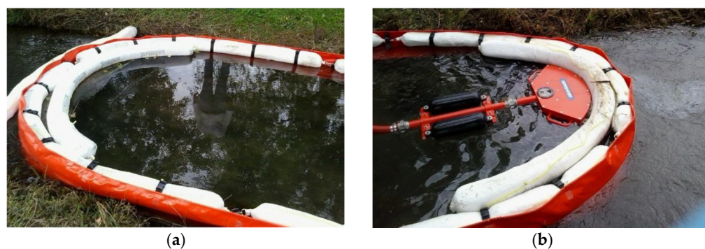
Figure 6. Example of a polypropylene boom (a) and oil recovery skimmer (b).
