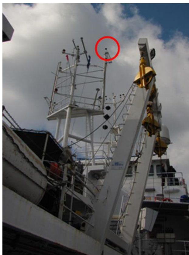
Figure 1. GNSS antenna and its installation on the Urania ship.
