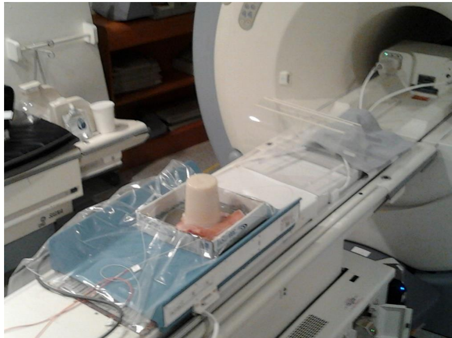
Figure 2. The realized configuration: the daily quality assurance (DQA) phantom over a skin portion. Although barely noticeable, the gel pad was placed under the skin to ensure acoustic coupling between the ExAblate bed and skin. In the left area of the image, the two interferometric probes are visible.
