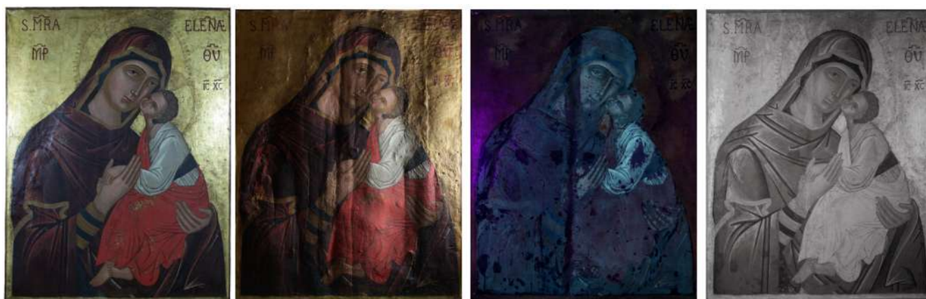
Figure 1. The Icon Madonna dell'Elemosina (Biancavilla (CT), Italy). From (left) to (right): photo in diffused vis light; vis grazing light; UV fluorescence; IR reflectography.
