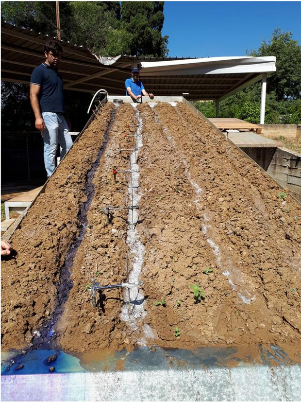
**Fig. 5** View of the rills after spraying the surface of the channels with a vinylic glue
