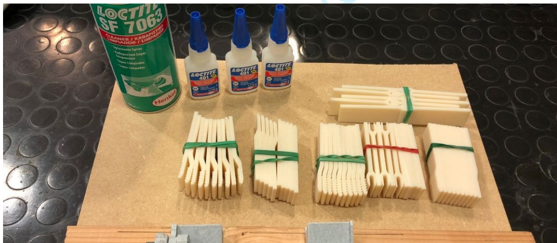
16 17 18 19 20 21 22 23 24 25 26 27 28 29 30 31 32 33 34 35 36 37 38 39 40 41 42 43 44 45 46 47 48 49 50 51 52 53 16 54 17 55 18 56 19 57 20 58 21 59 22 60 23 Figure 4 – 3D printed specimens before bonding with Loctite 401
