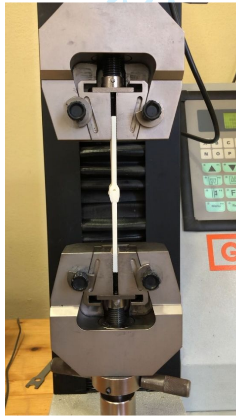
Figure 6 – Experimental tensile test on Double Lap bonded joints
