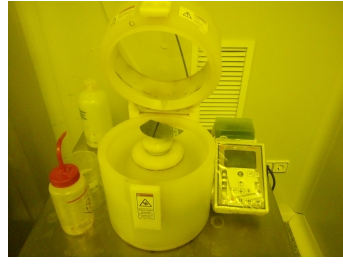
Figure 3.4: Spin coating equipment. Using a Laurell Technologies Corporation, WS-650-23 model.
