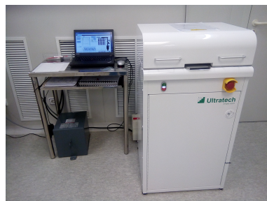
Figure 3.3: Atomic Layer Deposition (ALD) equipment. Using Ultratech Savannah ALD System.
