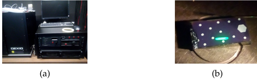
Figure 3.9: (a) PV Measurements QEX10 Quantum Efficiency measurement system and, (b) monochromatic beam illumination over one sample.
