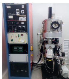
Figure 3.1: Thermal evaporator equipment. Using a Leybolds Systems, Turbovac TMP 600C and a Alcatel HI2000 for its alimentation.
