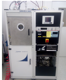
Figure 3.2: RF Sputtering equipment. Using a Advanced Energy, Cesar RF Power Generation and a Leybolds Systems, UNIVEX 350G glovebox system.
