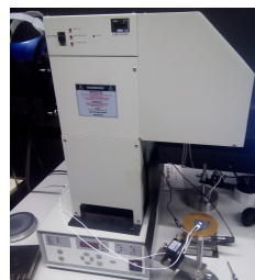
Figure 3.8: Solar simulator NEWPORT 94081A Class ABB Solar Simulator.
