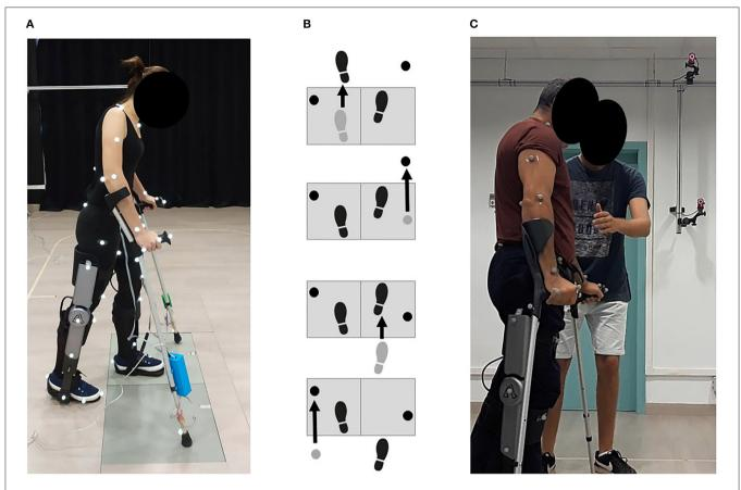
FIGURE 2 | (A) Healthy subject experimental data collection. She walked in the transverse direction with respect to the force plates and used instrumented crutches. Three different trials were performed: one without knee flexion-extension assistance (locked knee), and two with different levels of maximum knee flexion during swing.
