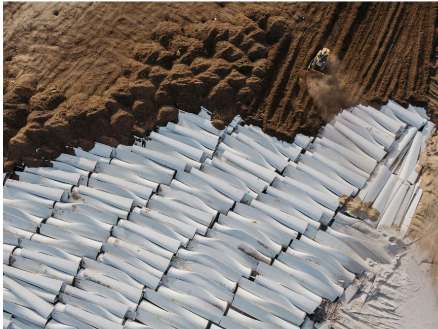
Figure 3. Fragments of wind turbine blades in Wyoming. Source: C. Martin
