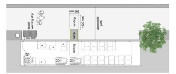
Figure 15. The layout of tactile surfaces on a bus stop platform in Dubai. Source: Own elaboration
