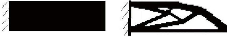
Fig. 11: Initial (left) and optimized (right) structure of a cantilever beam using a topological optimization algorithm (Chen et al., 2018)
