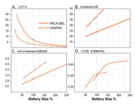
**Figure 11.** (**A**): LLP for varying battery bank sizes; (**B**): Investment for varying battery bank sizes; (**C**): Unit investment for varying battery bank sizes; (**D**): LCOE for varying battery bank sizes (present situation is shown with a dot). Solid line is for VRLA-GEL; dashed line is the projected behavior for LiFePO4 technology.
