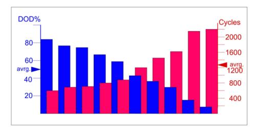
Figure 10. Frequency distribution of DOD and corresponding expected battery duration in cycles.
