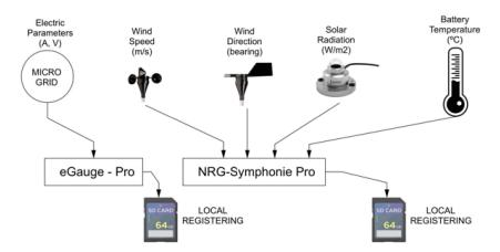
Figure 4. General setup for data collection and registering.
