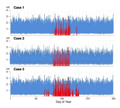
**Figure 13.** Annual profiles for load (in blue) and capacity shortage (in red) for HOMER-optimized cases 1, 2, and 3.
