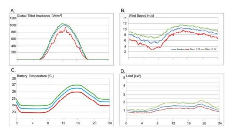
**Figure 6.** (**A**): Hourly profiles of GTI; (**B**): Hourly profiles of wind speed; (**C**): Hourly profiles of battery temperature; (**D**): Hourly profiles of load.
