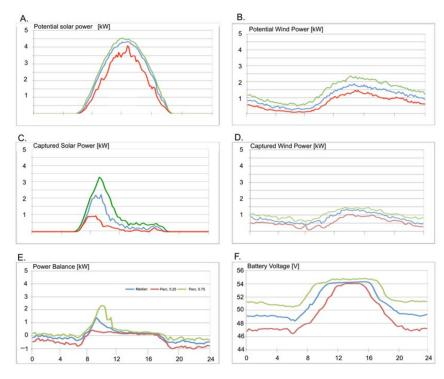
**Figure 7.** (**A**): Hourly profiles of potential solar power; (**B**): Hourly profiles of potential wind power; (**C**): Hourly profiles of captured solar power; (**D**): Hourly profiles of captured wind power; (**E**): Hourly profiles of power balance; (**F**): Hourly profiles of battery voltage.
