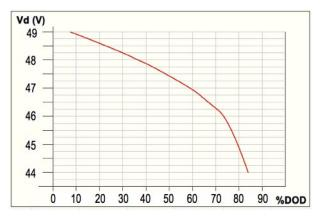
Figure 9. Battery bank voltage measured in discharge and corresponding DOD.
