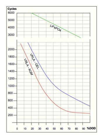
Figure 8. Battery duration to 60% SOH in charge–discharge cycles for different DOD and technologies.
