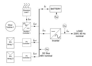
Figure 3. Scheme of Laguna Grande hybrid microgrid.
