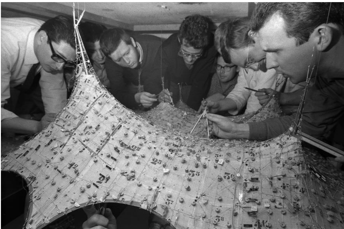
FIG. 3.18_ Measuring model of the German Pavilion at the Montreal World's Fair Expo '67.
