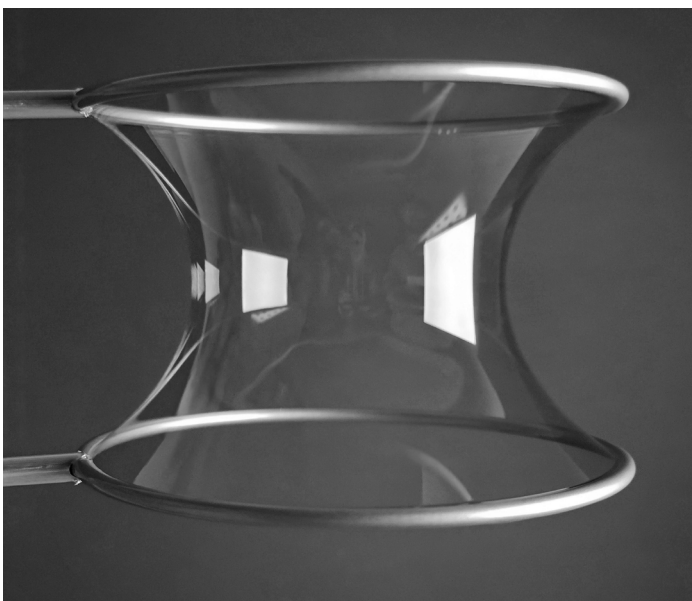
FIG. 3.31_ Soap film catenoid.
