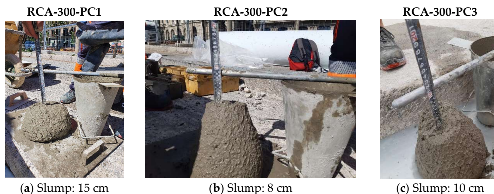
Figure 5. On-site slump test determination.
