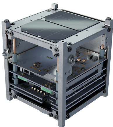
(a) Basic 1U Cubesat structure. Source: Cubesatworld [5].
