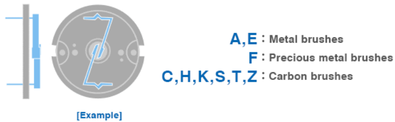
Figure F.3 Motor brush construction. Source: Mabuchi Motors [92].
