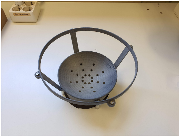
(a) Air bearing structure. Source: Own.
