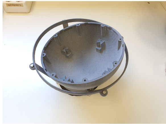
(b) Air bearing with CubeSat mount. Source: Own.
