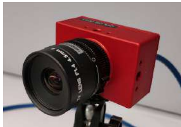
Figure 3.3: DAVIS 346 event-based camera from iniVation.
