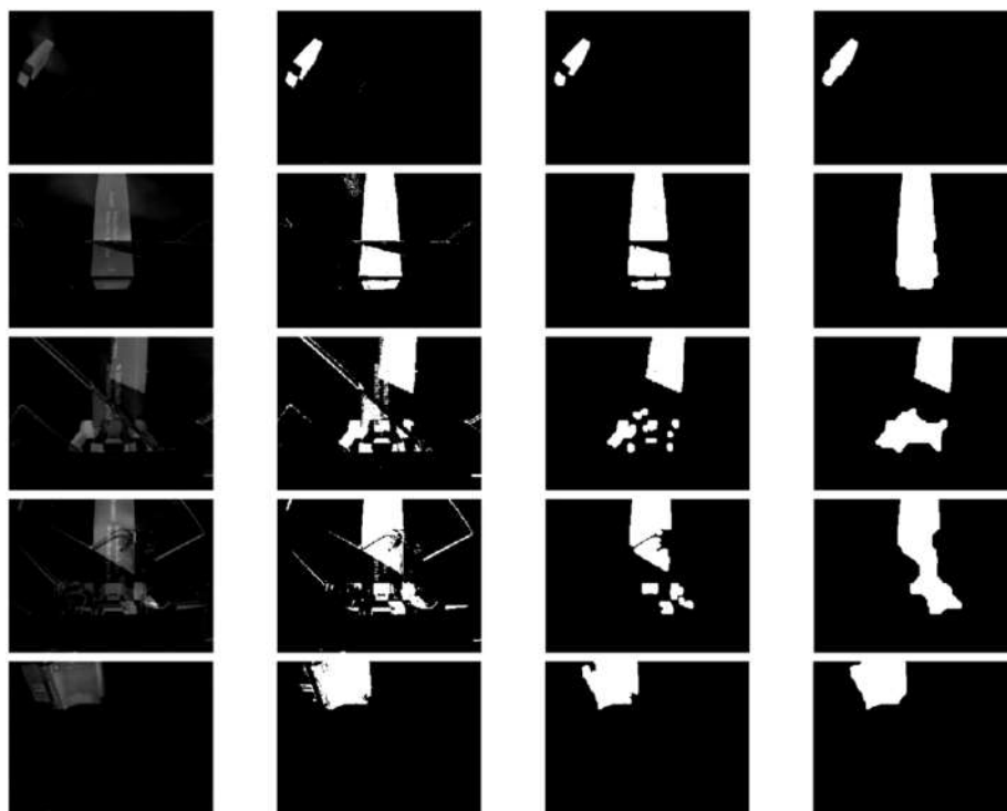
Figure 5.15: Sequence of images with the steps to generate the variable mask. The first column is the subtraction between the empty and with object sequence. The second is generated from the first by computing a binary image. Then, in the third, an opening operation is done and in the fourth a closing one is performed to generate the final mask.
