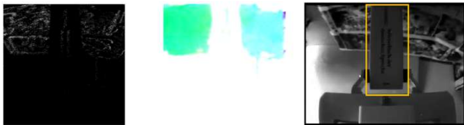
Figure 5.30: Event images (first column), motion flow estimation using optical flow (second column) and grayscale frames (third column) for the sequence in Figure 4.12.
