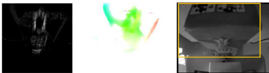
Figure 5.28: Event images (first column), motion flow estimation using optical flow (second column) and grayscale frames (third column) for the sequence in Figure 4.11.
