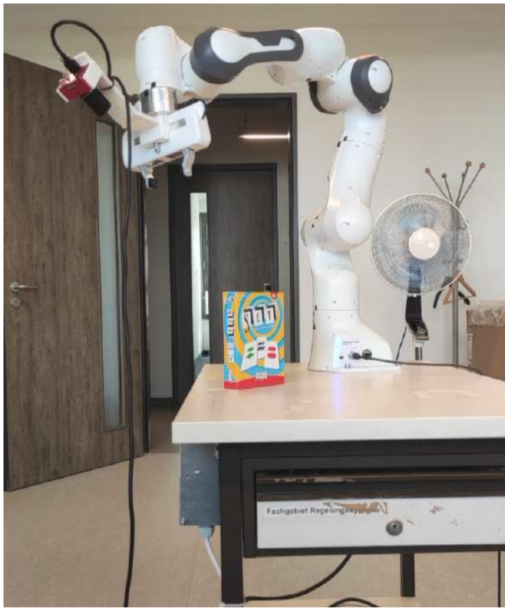
Figure 3.9: Experiment setup: robotic arm, gripper, event-based camera and its mount.
