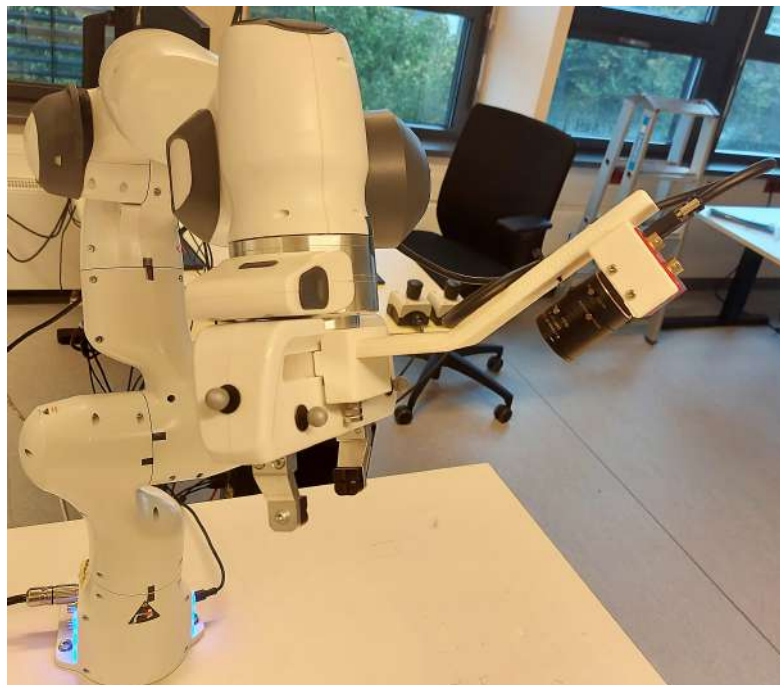
Figure 3.6: 3D printed mount assembled with the robotic arm and event-based camera.
