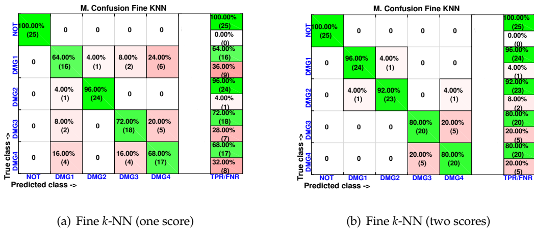
FIGURE 2.20: Confusion matrix using fine k -NN when the feature vector is formed by the first principal component (left) or by the first two principal components (right).
