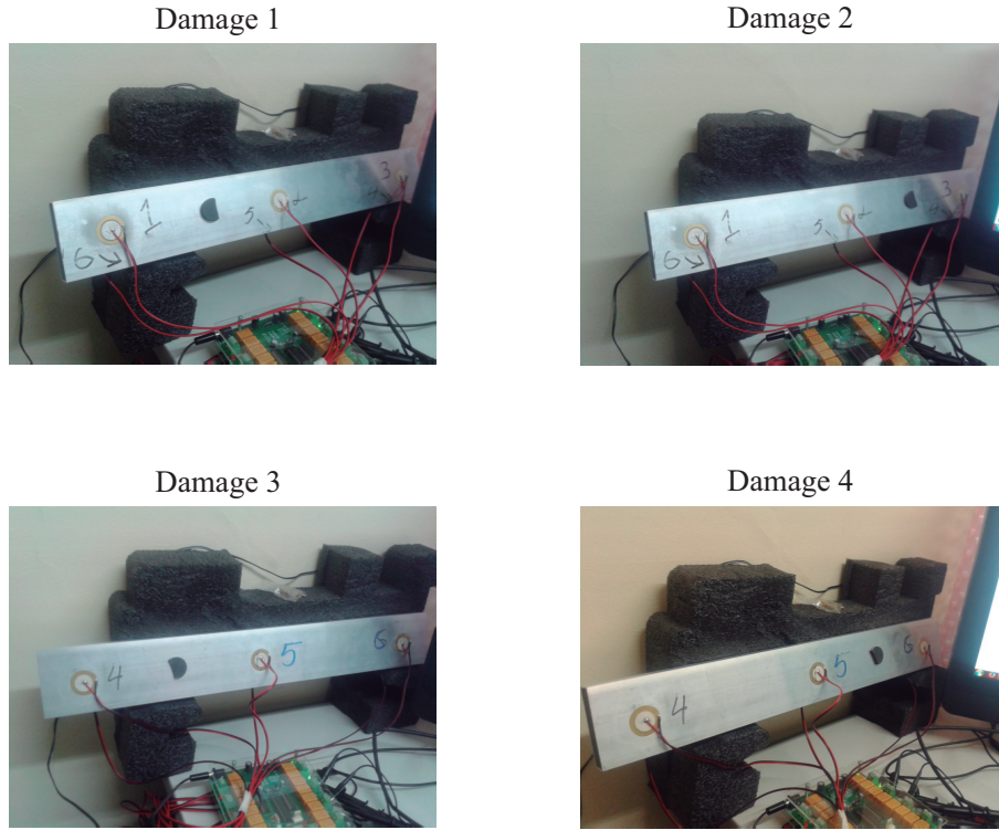
FIGURE 2.12: Aluminum rectangular profile instrumented with 6 piezoelectric sensors.
