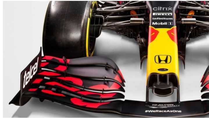
Figure 37. Red Bull 2021 front wing. (Source: [2])
