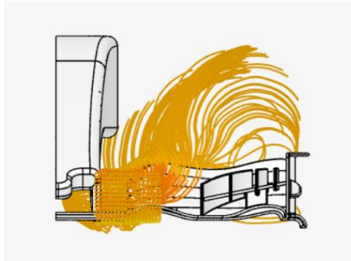
Figure 58. Particle traces creating vortices.
