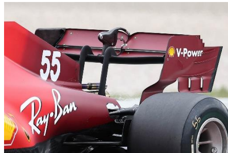
Figure 3. Ferrari SF-21 rear wing 2021. (Source: [2])
