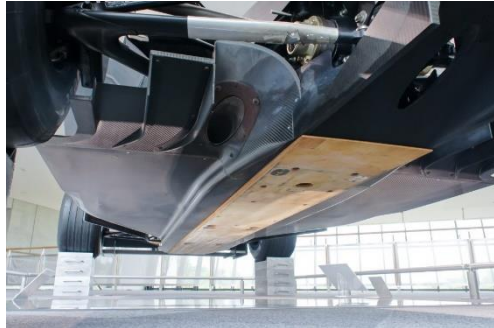
Figure 8. Mercedes AMG floor's car. (Source: [3])
