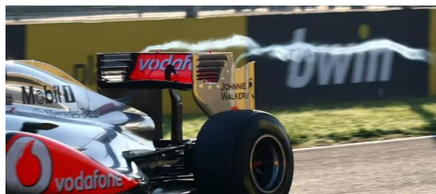
Figure 7. Vortices creation at the end of the endplates. (Source: [4])
