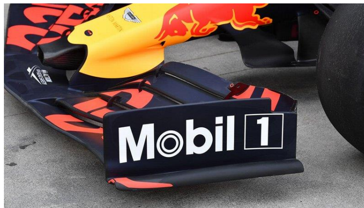
Figure 42. RedBull F1 team's footplate. (Source: [8])
