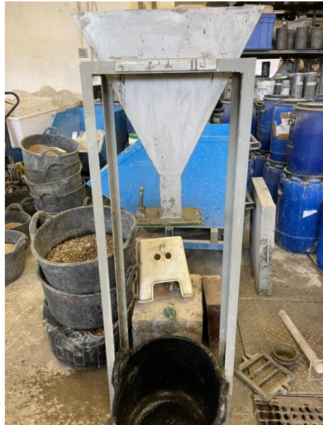
Figure 5. V-Funnel test equipment.
