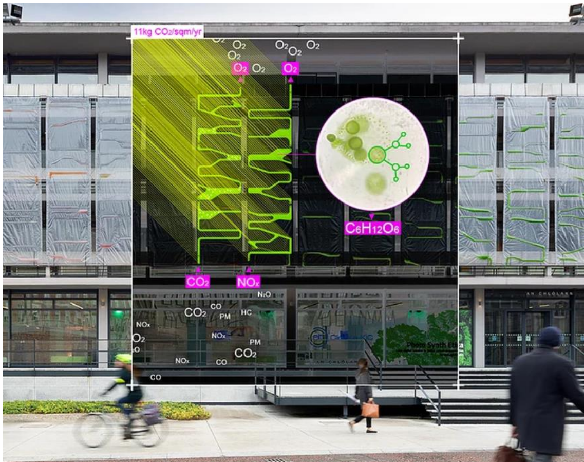
Figure 5.7: Photosynthetic building cladding system mechanism, Dublin, 2018.
