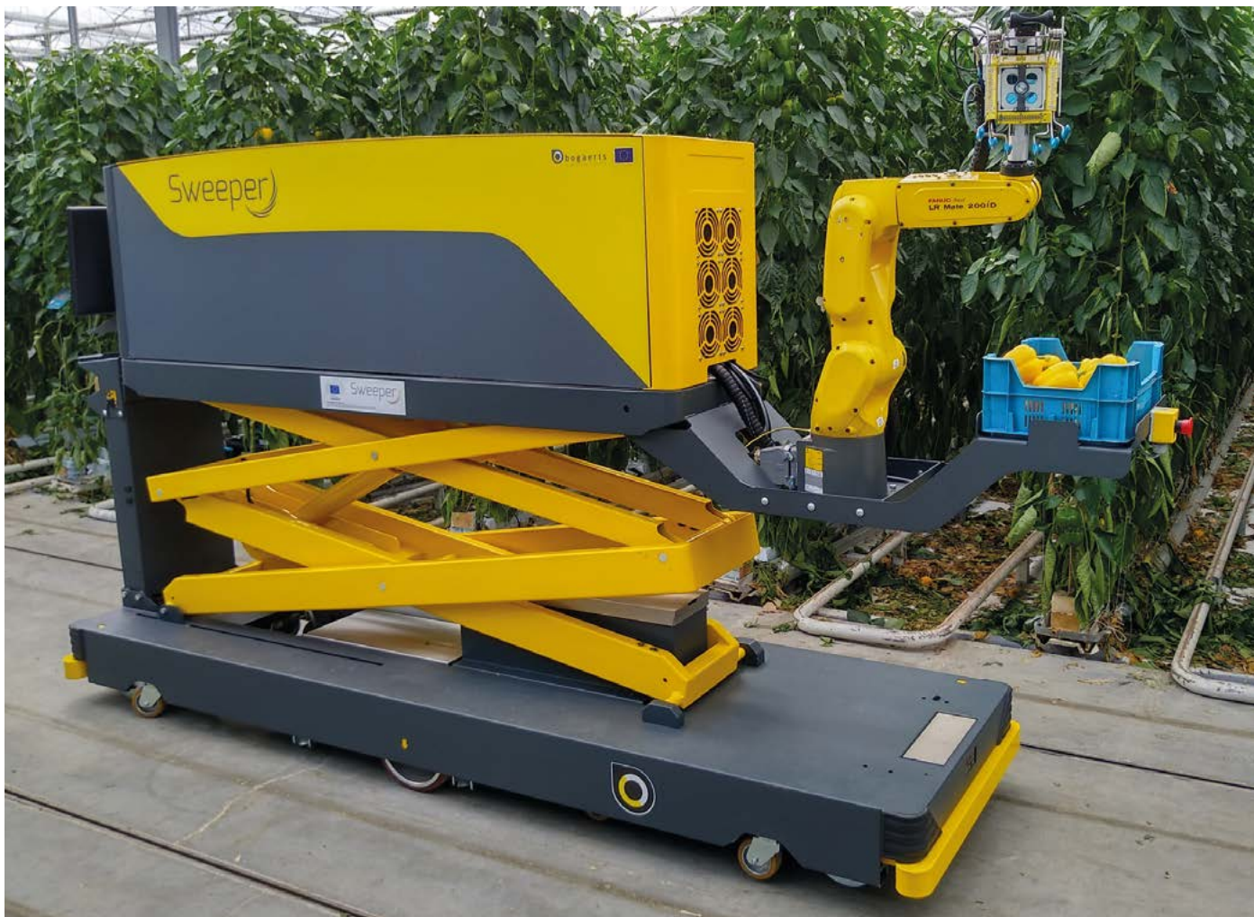
Robot for automatic harvesting of garden produce depending on its ripeness, developed as part of the SWEEPER project funded by the European Union's Horizon 2020 programme. Photo: www.sweeper-robot.eu
