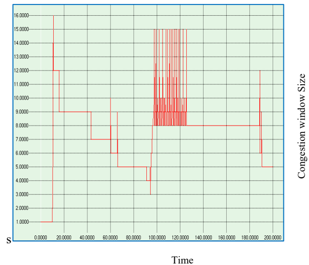
Figure 13. How AVGR controls the cwnd size when the burst contention probability is 10^{-4}
