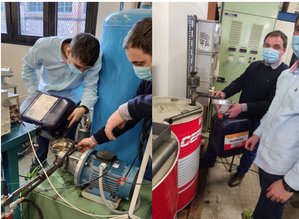
Figure 32 Filling the hydraulic oil in the tank
