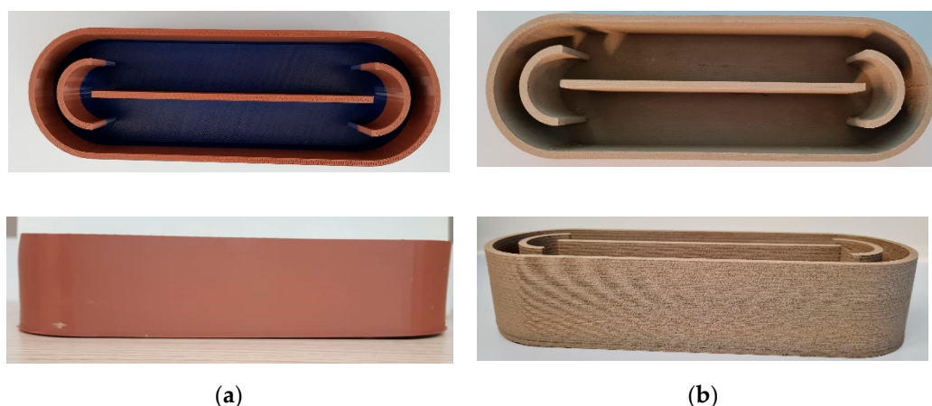
Figure 6. Picture of the 3D-printed race pond reactors (RPRs): PLA (a) and Timberfill® (b).
