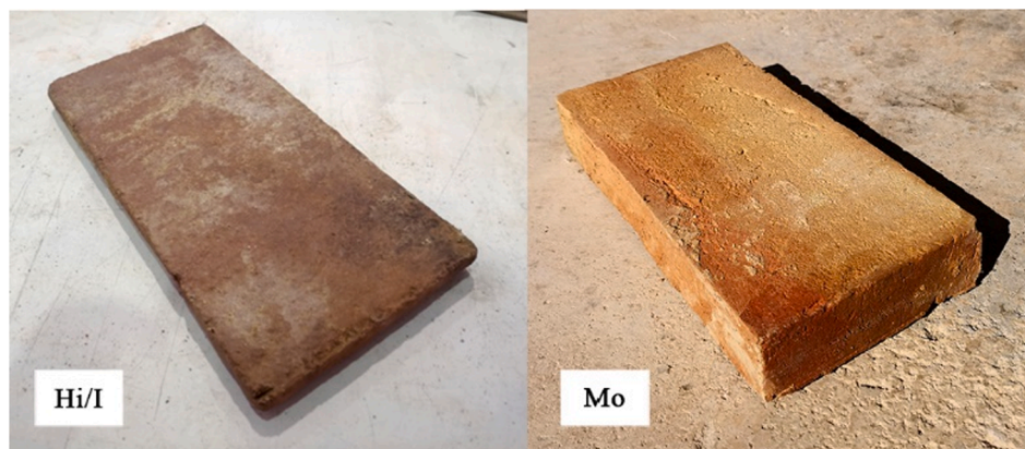
Fig. 2. Historical solid clay tile from industrial building (Hi/I) (left) and modern handmade solid clay brick (Mo) (right).
