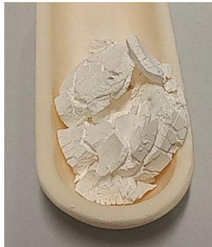
Figure 63 – \text{Ca(OH)}_2 sintered pellets once taken out of the oven.
