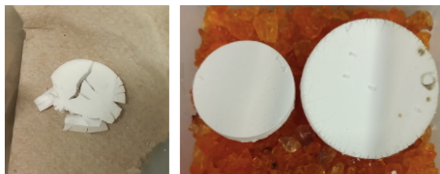
Figure 22 – Sintered CIP samples breaking (left) and enlarging after reacting with water vapor in the air in comparison with unreacted sample (centre tablet).
