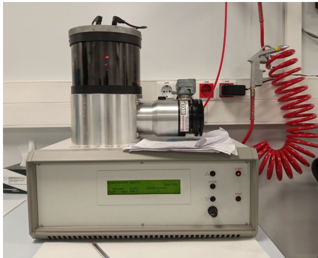
Figure 18 – Carbon Coating equipment for SEM analysis.
