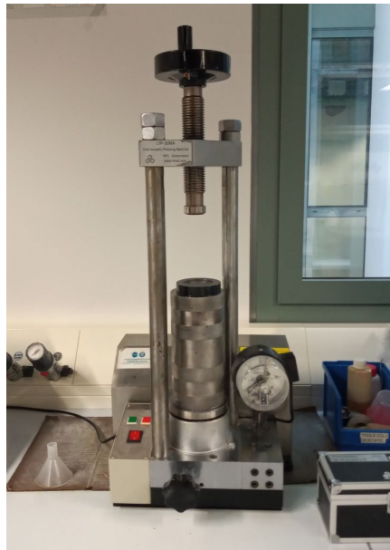
Figure 23 – CIP machine used in this Bachelor's project.
