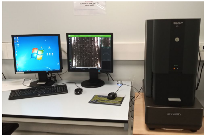
Figure 17 – SEM equipment used in this Bachelor's project.
