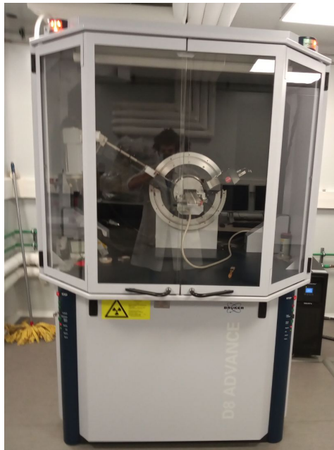
Figure 20 - D8 Advance D83 EDX equipment used in this Bachelor's project.
