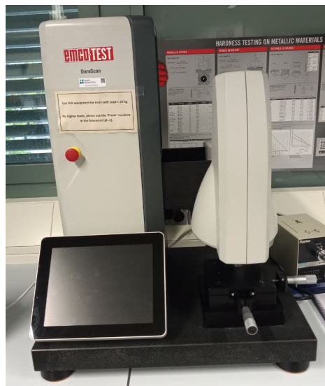
Figure 27 – DuraScan 65 Vickers microhardness equipment used in this Bachelor's project.
