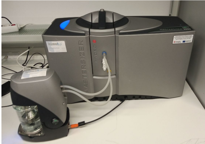
Figure 21 – Mastersizer 3000 Hydro EV laser diffraction equipment used in this Bachelor's project.
