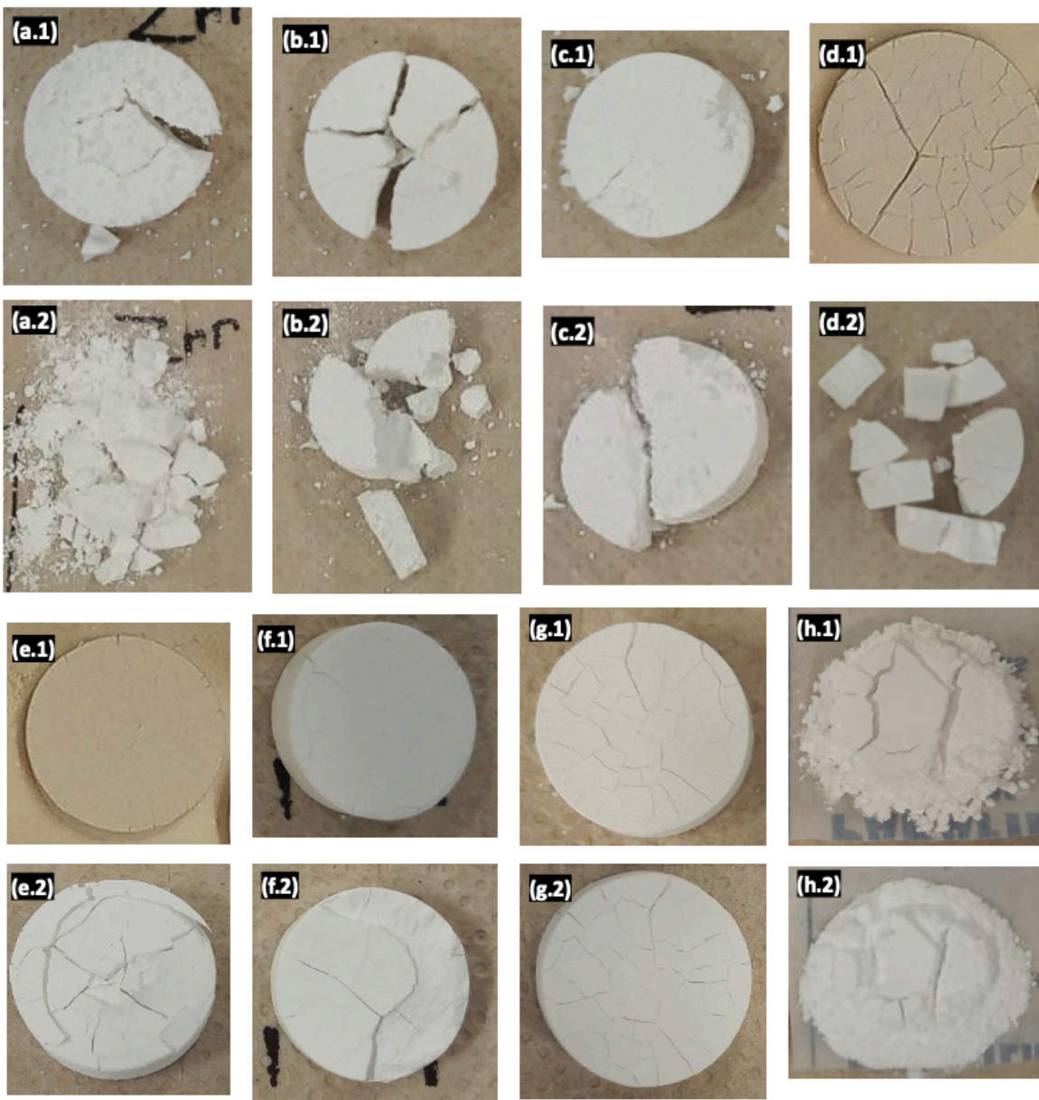
Figure 61 – Images of (a) Zr 1/10, (b) Zr 2/10, (c) Zr 3/10, (d) Al 1/10, (e) Al 2/10, (f) Al 3/10, (g) Al 4/10 and (h) CaO pellets sintered after (.1) 3 days and (.2) 7 days left in contact with air.
