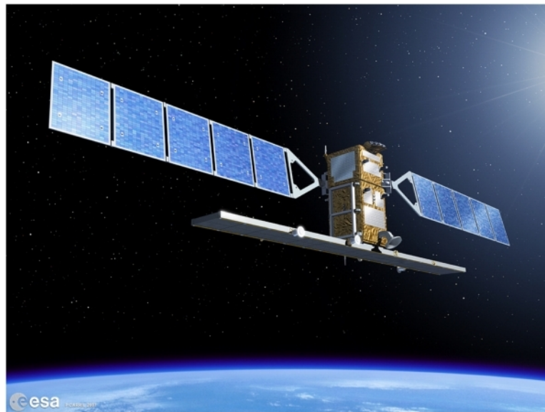
Figure 2.2: Satellite mounted SAR, Sentinel-1 by ESA
